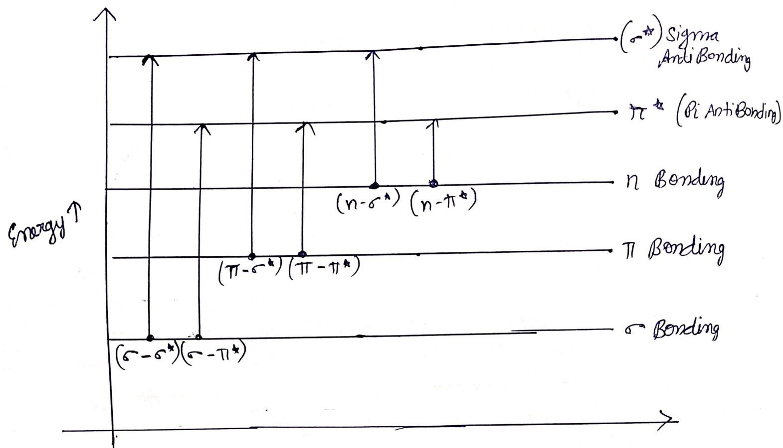
In given Representation, different Bonded compounds Absorb energy and gain different Transition States.
